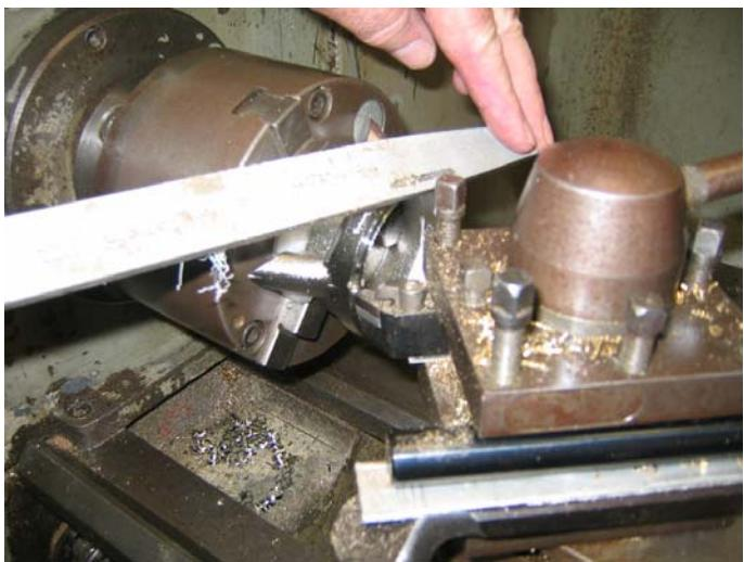
Remove aris from outer edge while Lathe is running with file
