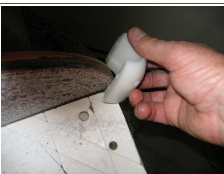
Grinding off the inner corners to enable easy assembly subsequent assembly.
