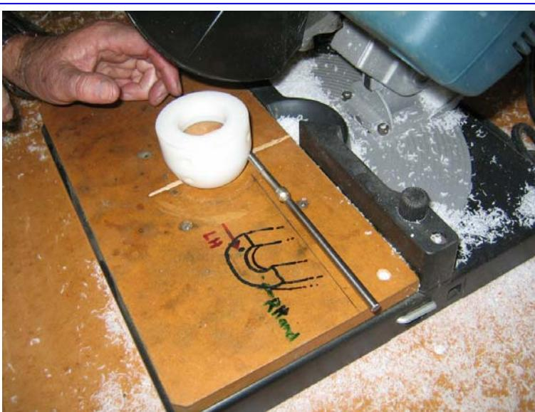
**Align tool with mark to ensure cut is at right angles to bolt holes**
