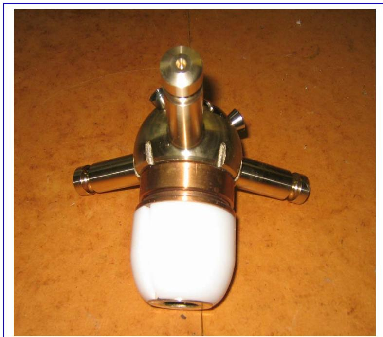
The jig is threaded and fits over the Boss to be expanded by unwinding the two halves until a snug fit between the blade carrier and the nose cone which is held manually in place
