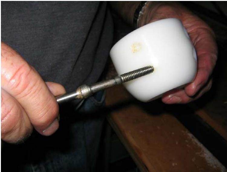
**Insert the tool into the lower 1/4" UNC thread as shown.**
