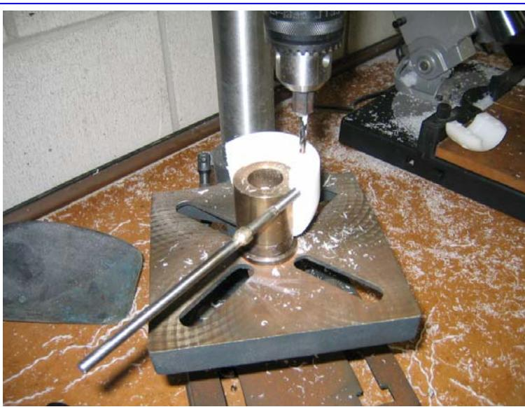
Mount on jig to bore and recess spring hole.
