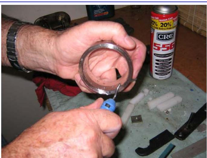
Deburr inside edge with deburring tool
