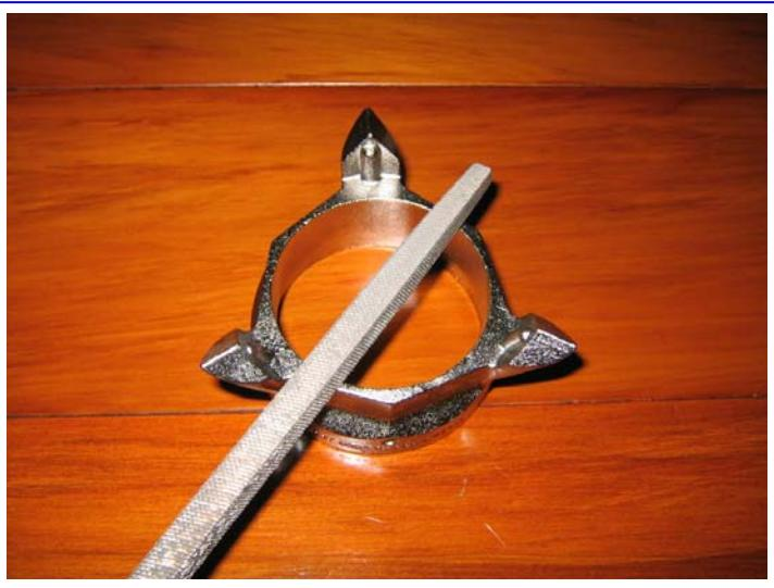
Check the inner corner of the Tripod to ensure nothing protrudes that could impact upon a flush fit against the blade carrier
